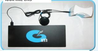
The lights on the MCU will blink RED when the button trigger is pressed and blink when the tap mat is touched.
