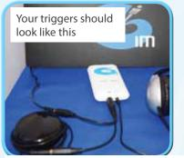
The lights on the PPU will blink **RED** when the button trigger is pressed and blink **WHITE** when the tap mat is touched.
