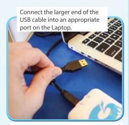
The plug will only fit one way, do **NOT** force the USB cable in the wrong way!
