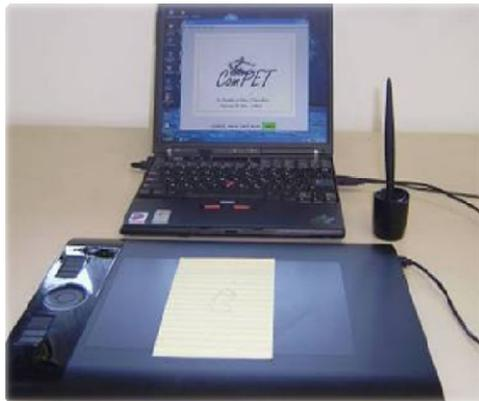
Fig. 1. Computerized penmanship evaluation tool (CompPET) – including a digitizing tablet and on-line data collection and analysis software.
