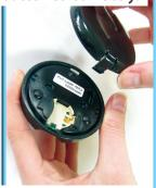
Squeeze the pressure clips to remove the cover from the button trigger
