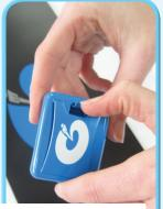
Remove the transmitter from the tap mat & press clip to open the cover
